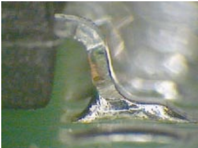
Figure 5-12 SnPb Solder; No Clean Process
